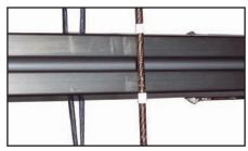
IMPORTANT: LUBRICATE THE STRING SERVING AND RAIL AT THIS TIME. FAILURE TO DO SO WILL RESULT IN EXCESS FRICTION, THE STRING SERVING BURNING AND WEARING OUT PREMATURELY
