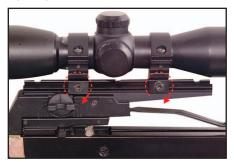
**Step 3:** Tighten the locking nuts using a screw driver.
