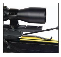
It is **IMPERATIVE** that the bolt is seated ALL the way back with the half moon nock cradled against the string. If this is not done the string may jump or go under the bolt – which would be equivalent to dry firing the bow (Firing without a bolt – this would void your warranty and damage could occur)
