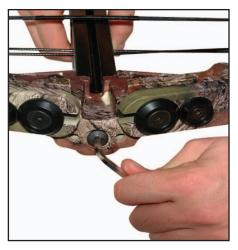
**Step 3:** Position the riser assembly and the body/stock together and prepare the nose bolt and washer for installation. Simply push the two pieces together so that they are properly aligned and use the Allen key to tighten the nose bolt. The stock/body and riser will cinch together as the nose bolt is tightened. Continue to tighten until the two pieces are securely tightened.
