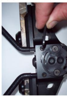
**Step 5:** Attach the quiver bracket with latch onto the quiver using the 2 wood screws. You will need a Phillips screwdriver to accomplish this. The latch is shown in the open position ready to mount the assembled quiver onto the crossbow.
