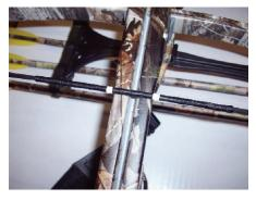
IMPORTANT: LUBRICATE THE STRING SERVING AND RAIL AT THIS TIME. FAILURE TO DO SO WILL RESULT IN EXCESS FRICTION, THE STRING SERVING BURNING AND WEARING OUT PREMATURELY
