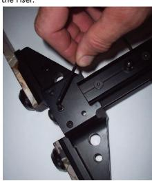
**Step 3:** Attach quiver mount to the underside of the riser using 2 counter sink allen screws and wrench provided.
