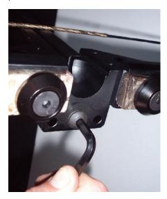
**Step 2:** Flip the crossbow over and secure the nose bolt from potentially loosening by tightening the grub screw on the center of the underside of the riser.
