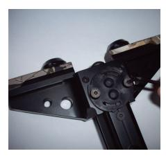
**Step 4:** Insert Foot stirrup into riser. With the crossbow still flipped over insert the foot stirrup into the riser with the two notched areas facing toward the grub screws shown below being tightened. The grub screws may need to be loosened slightly to be able to properly insert the foot stirrup.
