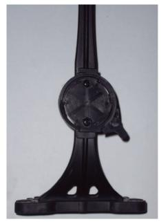
**Step 6:** Attach the quick detach quiver to the quiver mounting bracket using a twisting motion. The quiver should be at a diagonal angle in order to properly seat on the quick detach bracket prior to twisting into the fixed position.
