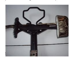
**Step 7:** Attach the padded shoulder sling to the crossbow. Loosen the thumb screw on the sling swivel so that the swivel may be attached to the sling studs located on the underside of the crossbow stock.
