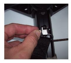
Tighten thumb screws securely on both swivels.
